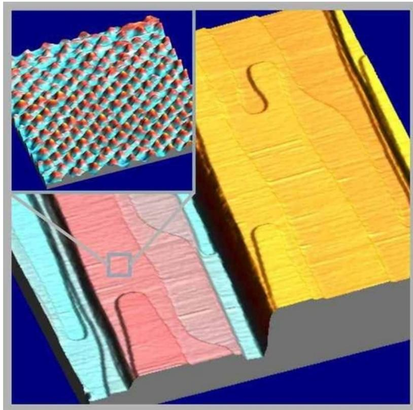
**Figure 1:** KBr(100) under ambient conditions. The inlay shows the atomic structure of the sample.
